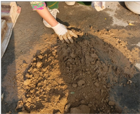
Figure 2 Manual Filling and Compaction of the Homogeneous clay, Treated Wastewater Mixture into
