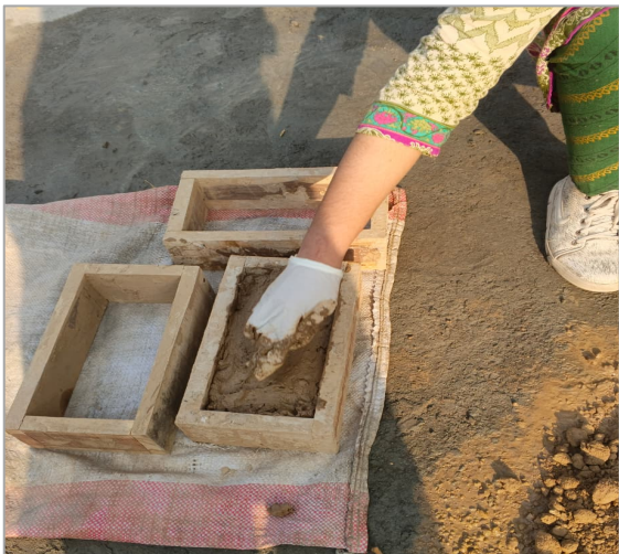
Figure 2 Manual Filling and Compaction of the Homogeneous clay, Treated Wastewater Mixture into
